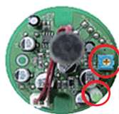
Variable Resistor (sensitivity adjustment)
