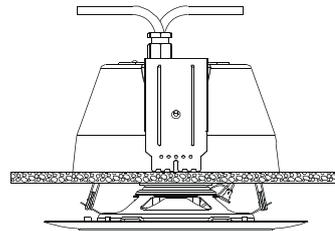
**10)** The fire dome should be firmly secured into the ceiling.
