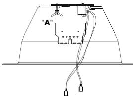
1) Remove the wing nut "A" located on the inside of the fire dome.
