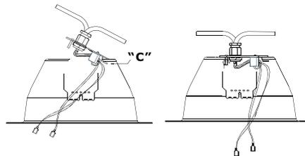
3) Gland the installation cable into the termination plate using suitably rated 20mm glands. 2 gland entries are provided for "loop in"/"loop out" termination if required.
