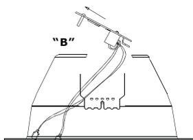
2) Lift the termination plate upwards & away to separate it from the fire dome "B".
